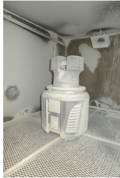
Fig. 11 APDIS after IP5X test.
