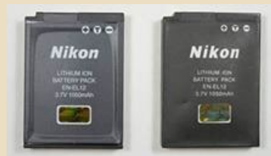
An example of a genuine Li-ion Rechargeable Battery EN-EL12 (left) and a counterfeit (right)
