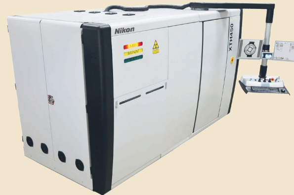
XT H 450 X-ray and CT inspection system
