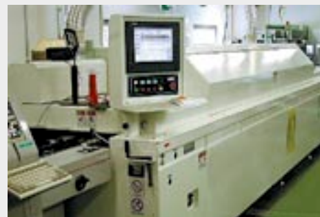
High-performance reflow furnace for lead-free soldering
